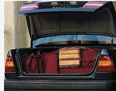
The 16.6 cubic-foot capacity (0.47 cubic meters) and low liftover height make the trunk easy to use.
